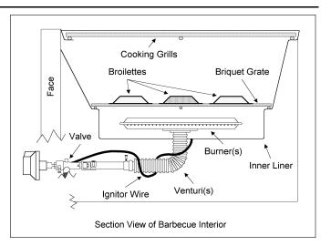
Replace the briquet grate and the broilettes. Distribute the broilettes evenly in the areas on the briquet grate surface above the flames from the burners. This will help the grill cook at an overall even temperature.
