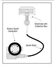
The ignitor sends a high voltage along the wire to the ignitor electrode inside the collector box. The collector box collects a quantity of gas, which a spark lights.
