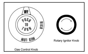
Your barbecue equipment will have several knobs on the face for controlling the gas and lighting the gas. The gas control knobs are labeled "PUSH TO TURN" in the center, "OFF" at the twelve o'clock position, "HIGH" at the three o'clock position and "MED LOW" at the six o'clock position. The rotary ignitor knobs are the smaller knobs with the directional arrows.
