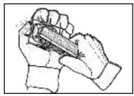
Next, remove and inspect the stainless steel Broilettes. Any badly deteriorated ones should be replaced. A light coating of rust is okay. Knock off any loose rust or deposits with a wire brush. You may wash them if you desire.
