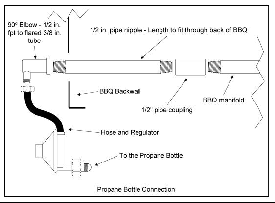
CAUTION: Propane, also known as LP, is a gas that is heavier than the surrounding air. You should not store your propane bottle in an area that can trap any escaping gas. This means that your storage area must be vented at the level of the base of your tank.
