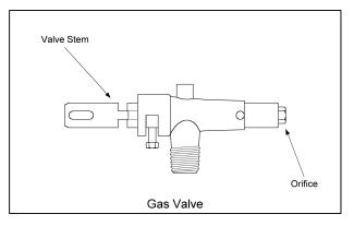
with a small piece of wire or toothpick. Re-install orifices and tighten.
