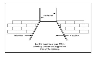
Fire Magic circulators may be use in multi-level fireplaces, combined in a single chimney (not a single flue). The standard rules that govern multi-level fireplaces and concerning flue offsets and heights apply.
